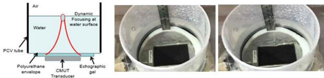
Fig 13: Acoustic fountain generated in HIFU mode with the first prototype of CMUT USgHIFU complete probe for the prostate (previous design in "real ring"). Schematic diagram and result. The acoustic fountain translates the ultrasonic power generation (qualitative) and the good focusing (quantitative: here at f = 52 mm).
